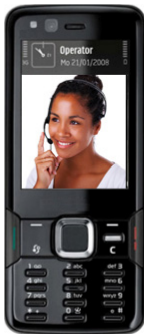
Figure 9. Video streamed back to the 3G mobile phone may be menu item selections, pictures, live streams, or any other video content the call center agent chooses.
